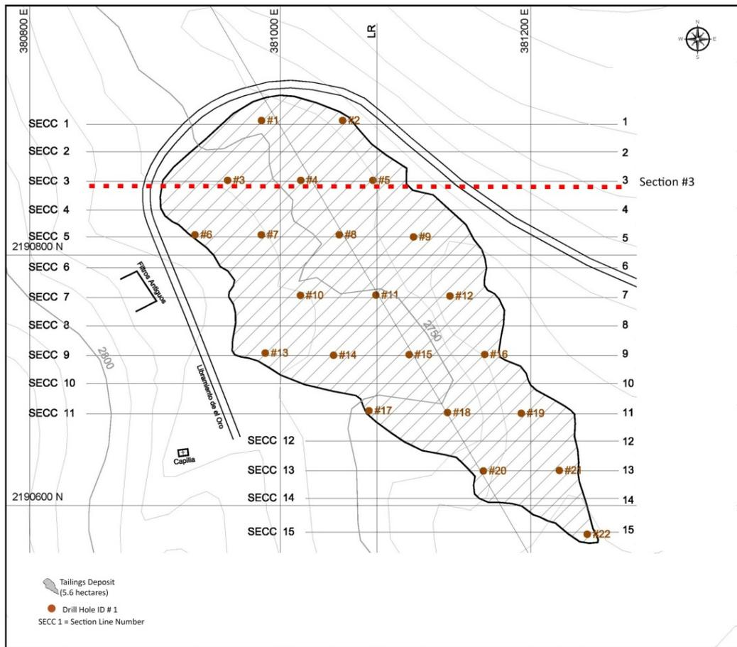
Figure 6.20: Plan Map Showing the 1990 Locations of the 22 Drill Holes by Luismin
