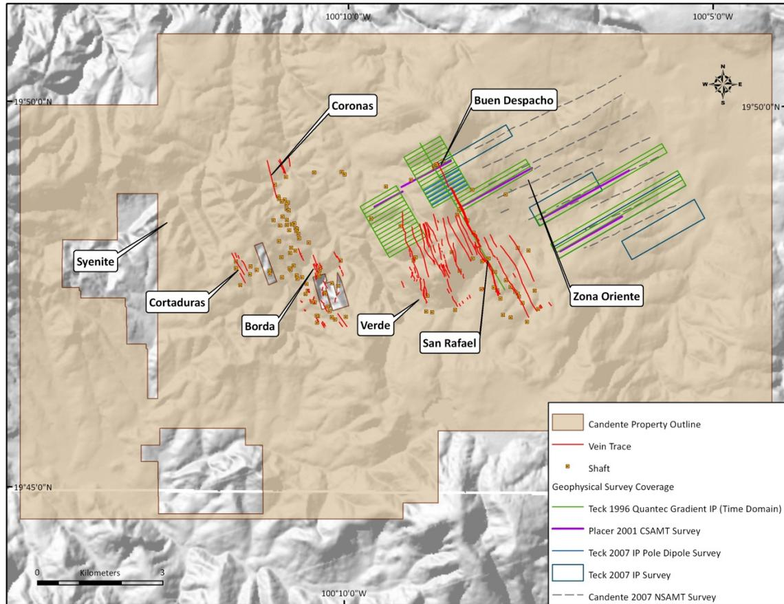
Figure 6.6: Distribution of the El Oro-Tlalpujahua Geophysical Surveys
