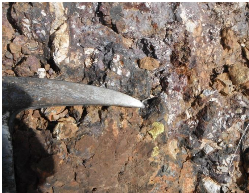
Figure 7.8. Mineralized breccia at the Cocula Project. View of mineralized breccia near hole RCC-2. Fragments of altered rock and vein material cemented by siliceous ferruginous matrix with abundant hematite.
