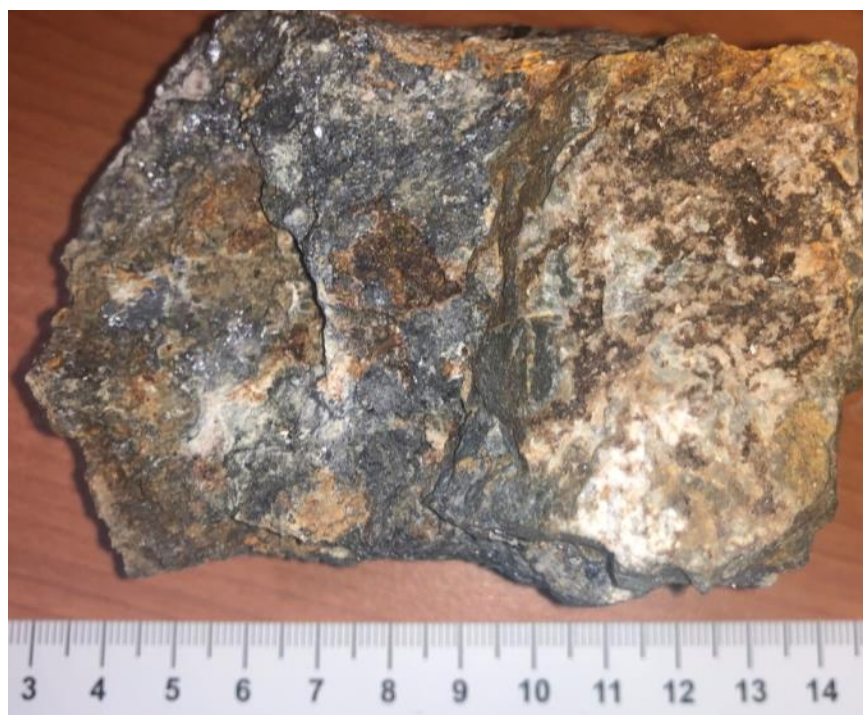
Figure 9.8. Galena-rich vein. Photo of sample 13371, a galena-rich epithermal vein from the Cocula Project. Scale in cm.
